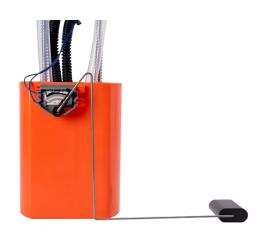
**STEP 12:** Install the new SureFlo sending unit into the tank as shown at right. See the application specific instructions below for proper clocking of your sending unit. Reinstall the locking ring.
