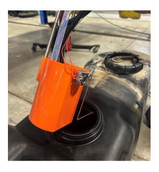
**Model Years 1999-2003 7.3L Powerstroke**: Orient the SureFlo sending unit to where the indented mark on the cap lines up with the notch in the tank flange as shown at right.
